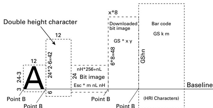
Figure 4-2 Mapping Positions for Print Data
