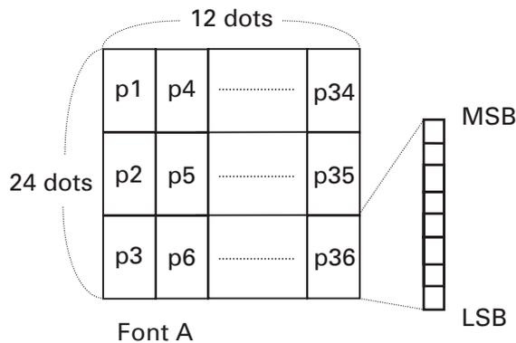
Create each data bit by setting “1” for a printed dot and “0” for an unprinted dot.
