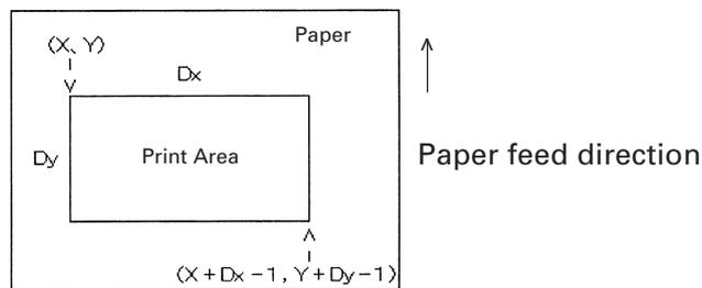
The printable area for this printer is approximately 80.078 mm (640/203 inches) horizontally and 117 mm (938/203 inches) vertically.
